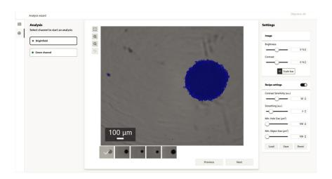
The CELLCYTE X offers a full solution to investigate spheroid formation, growth, and health in a streamlined manner. Optimize every step of your workflow including sample preparation, vessel type selection, study scheduling, image acquisition, real-time analysis, and data visualization with our latest spheroid software. Capture and quantify spheroid growth inside the incubator without disrupting ideal experimental conditions.
